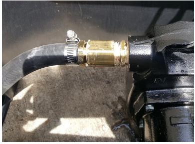
d. Slide hose clamps towards both ends of the hose, tighten with a screwdriver.
